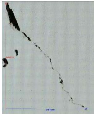
Figure 7: Destructive examination of Defect H in Specimen 4419-02 / BT01
