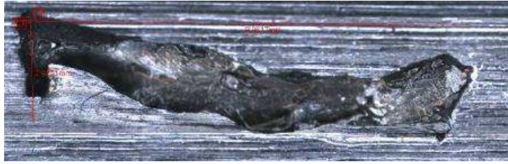
Figure 6: Destructive examination of Defect G in Specimen 4419-02 / BT01
